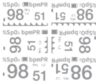
Press the power button continuously during the monitoring process. The data monitored and display method will be displayed cyclically on the OLED screen in two different ways (large fonts and plethysmograph) and in four directions, as shown in the illustration.
