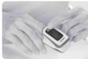
Insert a finger fully into the oximeter's measuring sections. Keep the surface of the nail pointing upwards and release the clip. Press the power button to switch on the oximeter.
