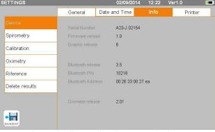
At this point, **spirolab** can use the connection via SPP (Serial Port Profile) protocol. For details on using the protocol, please contact the manufacturer.
